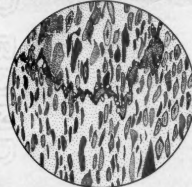
FIGURE 12. MUD PELLETS AND LAYERED OIDS IN CRYSTALLINE MATRIX Deformed normal to bedding which is studded with quartz grains and much contorted. Spec. 332, Conococheague limestone, 3 1/4 miles S. Carlisle, Pa. ac section, deformation 40 per cent.
